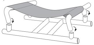
If you can't press the seat platform into the seat frame you can turn the assembly upside down (so that the fabric is on the ground) and stand on the seat rails. You can also use a rubber mallet.
